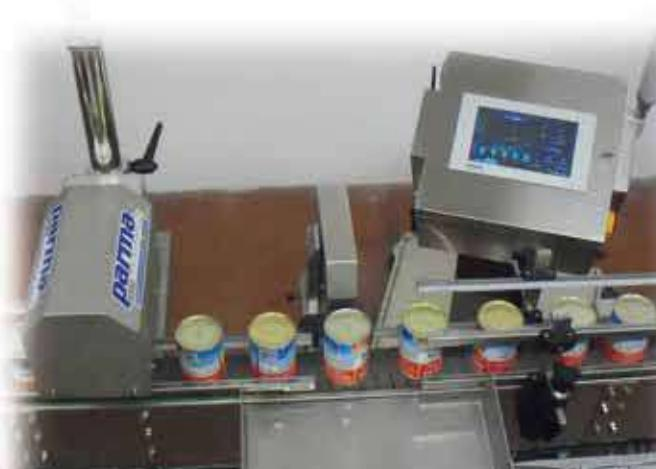
The ControlPressure checks the pressure (lid convexity) of aluminium cans in filling lines for flat products with liquid nitrogen dosing system. This same system may be used immediately after the seamer to check the good functioning of the dosing system (rough inspection), or at line end for making sure that the container still maintains the pressure and it is airtight after thermal treatments (precise inspection).
