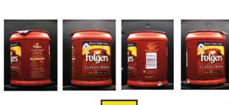
Seam inspection over the 360° with 4+1 cameras
