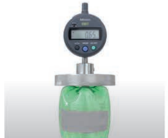
BASE CLEARANCE CHECK
